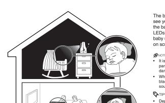
The baby unit has infrared LEDs that allow you to see your baby at night or in a dark room. When the baby unit detects low light levels, the infrared LEDs turn on automatically. The images from this baby unit is in black and white, and \*\* appears on screen.
