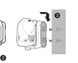
Place the baby unit on the wall mount bracket. Tighten the screw into the threaded socket at the bottom to secure the baby unit. Align the holes on the wall mount bracket with the screws on the wall, and slide the wall mount bracket down until it locks into place.
